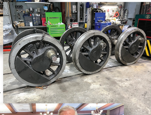
Ten wheeler #12's driving wheels out and on display during her tear-down at Tweetsie.
