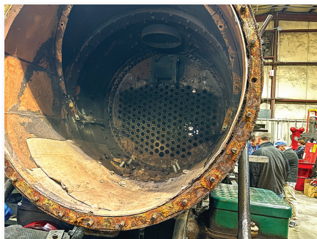
Engine 12's soon-to-be-replaced smokebox and boiler tubes. Photo by Chris Ford.
