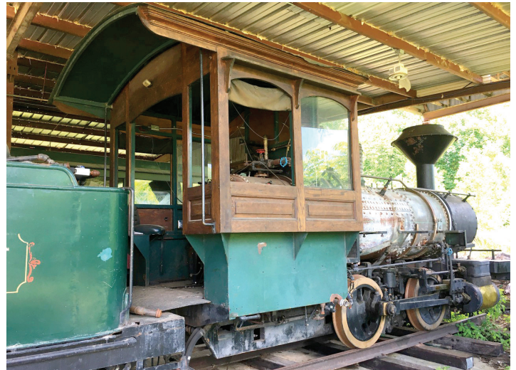
One of the two newly acquired Porter engines for the Doe River Gorge’s exciting new Christmas Train project. Both engines are scheduled for boiler replacement.
