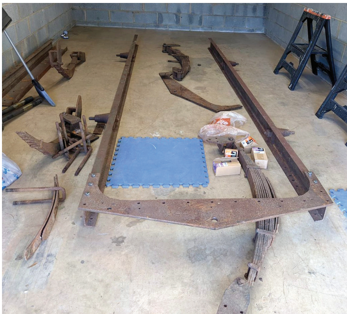
The reassembled frame of ET&WNC Motorcar #1 and some of its precious pieces await further attention in its newly prepared "shop". Photo courtesy of Matt Bumgarner.
